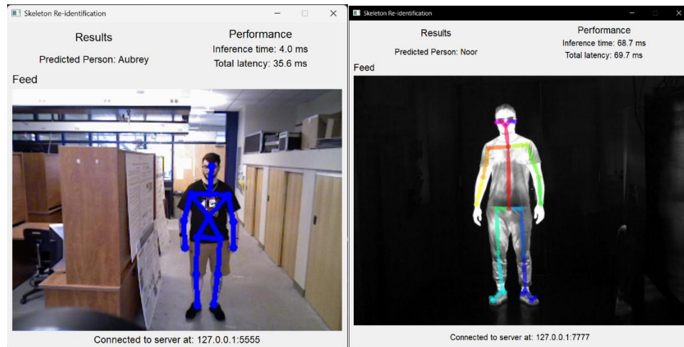
Figure 6: Tracked skeleton on PrimeSense and FLIR cameras respectively.
